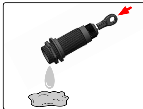
Drain the oil from the shock absorber.
